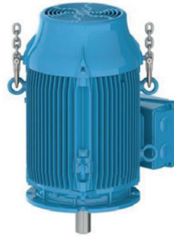
Figure 4.17 - Install the first pair of eyebolts
