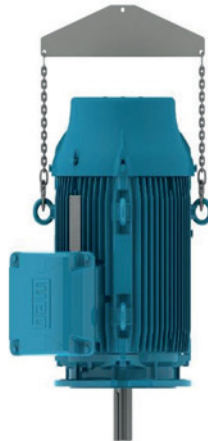
Figure 4.8 - Lifting of vertical mounted motors
