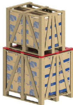
Figure 5.5 - Use of additional battens for stacking
