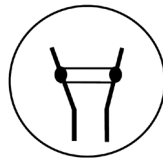
IEC 60947-5-1 Mechanically linked contacts
