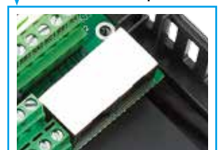
Dual RJ45 communication ports
