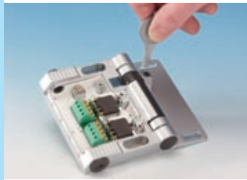
Setting the switching point with a special tool
