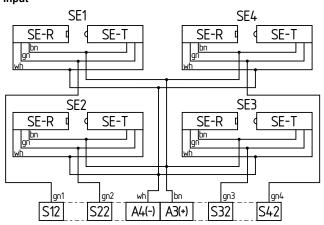
If less than 4 safety edges are connected, the following diagram must be observed. Unused inputs must be connected as shown.
