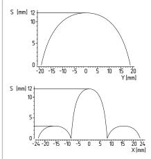
The axial misalignment (Y) is max.  $\pm$  18 mm. The height misalignment (X) is max.  $\pm$  8 mm. Avoid area of side lobes if lateral activated.
