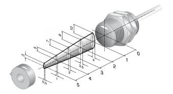
$s_{ao} = 5 \text{ mm}$ assured switching distance:
