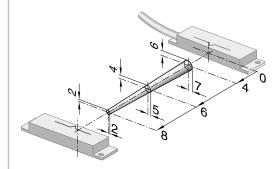
Assured switching distance:  $s_{ao} = 8 \text{ mm}$ Assured switch-off distance:  $s_{ar} = 18 \text{ mm}$
