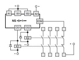
The NS •5••1••• version, in addition to maintaining the operating and safety characteristics of the NS series, allows control of **forcibly guided NC contacts of contactors or relays** controlled by the safety outputs of the switch itself. As an alternative to the relays or contactors you can use Pizzato Elettrica expansion modules CS ME-03 (see page 267). This check is carried out via the EDM input (External Device Monitoring as defined in EN 61496-1) of the switch.
