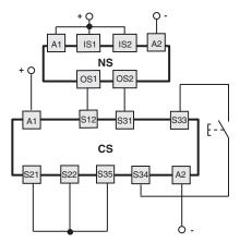
Connections with CS MF•••••, CS MP••••• safety modules
