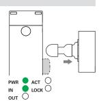
When the actuator leaves the actuation limit area, the device turns off the ACT LED and the O3 signalling output.
