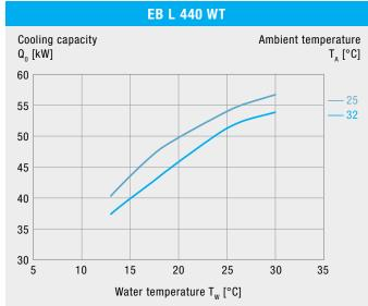
**EB 2.0:** The performance curves include standard pump losses and refer to operation at 50 Hz with water. Compared to values indicated for ambient temperature of 32 °C, capacity values will decrease by approximately 20 % (30 %) during operation at 40 °C (45 °C) ambient temperature.
