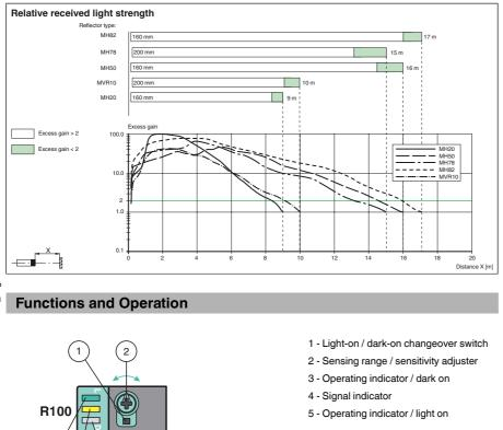
To unlock the adjustment functions turn the sensing range /sensitivity adjuster for more than 180 degrees.
