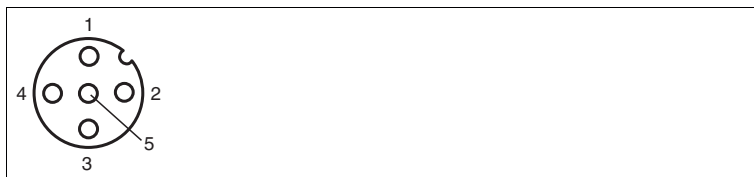
Pin assignment of the M12 socket for RS 232
