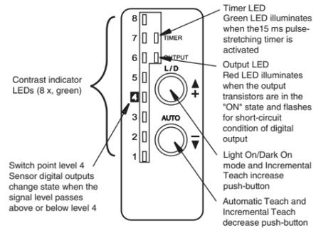
Figure 3. Push-buttons and Status Indication LEDs
