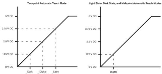
Figure 2. Digital Output Thresholds for Automatic Teach Modes
