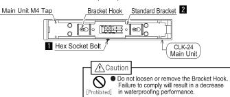
2 Attach the SZ320-KS to the main unit of LED Work Light. Attach an M4 screw to the "Model CLK-24(A)AG mounting hole" and "Main Unit M4 tap". Use a mounting torque of 1.4 N m
