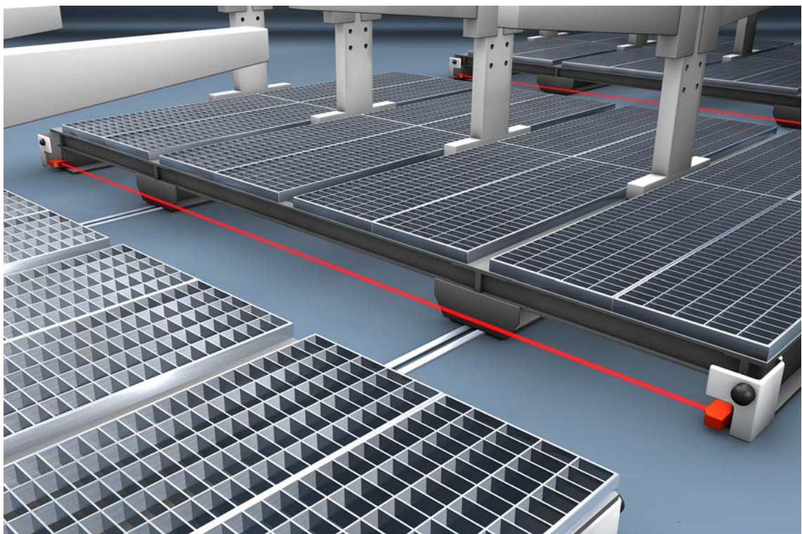
Figure 5.3: Foot-space protection on side-tracking shelves
