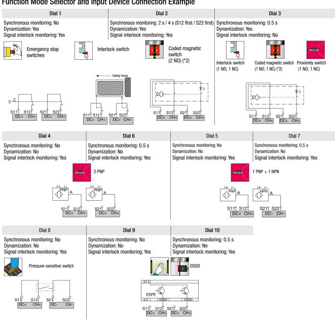
\*2: Connection examples for coded magnetic switches such as HS7A (IDEC) are also included on the instruction sheet, but certifications are not available.
