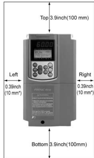
Figure 2.1 Mounting Direction and Required Clearances
