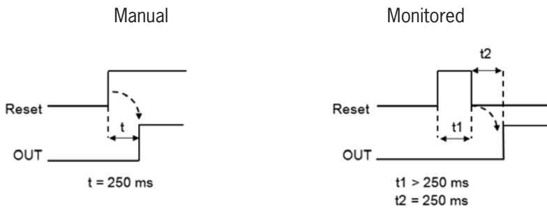
Figure 89: Interlock manual/monitored reset
