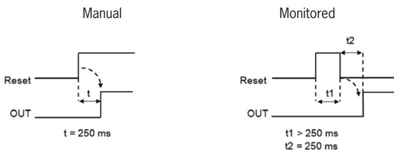
Figure 112: Pressure sensitive mat manual/monitored reset
