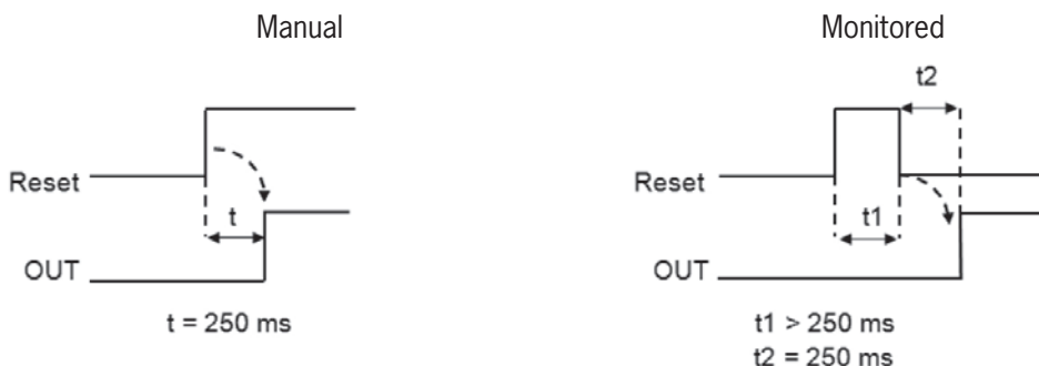
Figure 166: Guard locking logic manual/monitored reset
