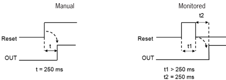
Figure 123: Semiconductor output manual/monitored reset
