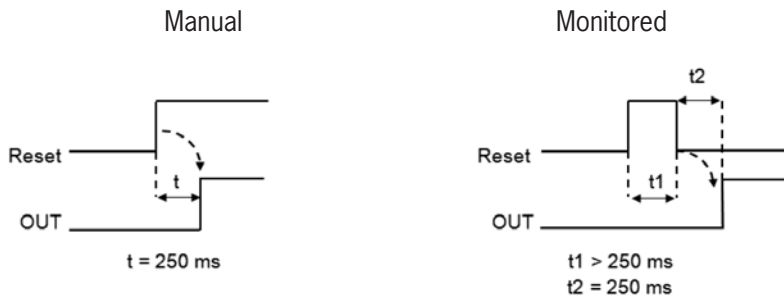
Figure 105: Light barrier manual/monitored reset
