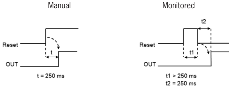
Figure 98: ESPE manual/monitored reset
