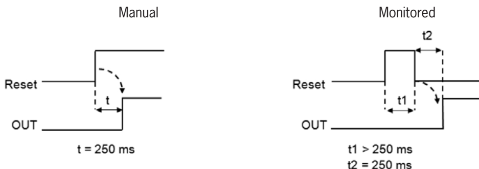
Figure 115: Switch manual/monitored reset
